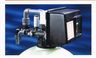
This range suits all sizes of domestic properties and small industrial sites, treating all the water from a borehole pump. They continually aerate the water in service and use air and water to backwash. This means they can cope with higher iron and hydrogen sulphide (rotten egg smell) levels, higher flow rates and use about half the service flow rate to backwash. As fully integrated filters they contain all the aerating and venting components.
